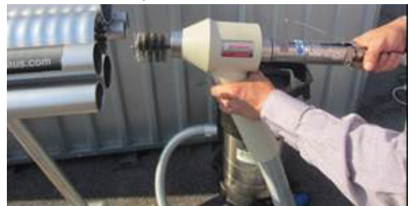
4) Y-piece and a vacuum cleaner avoid releasing of dust, e.g. if the suction fan has turned off
